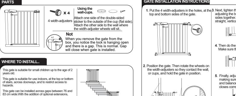
gaps up to 139 cm can be secured. Make sure the gate is installed on a flat, secure, strong surface.
